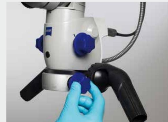
Figure 1.13 Adjusting the focus dial
