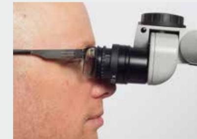
Figure 1.12c Viewing with eyeglasses: screw in the eyecups all the way (no silver ring visible)
