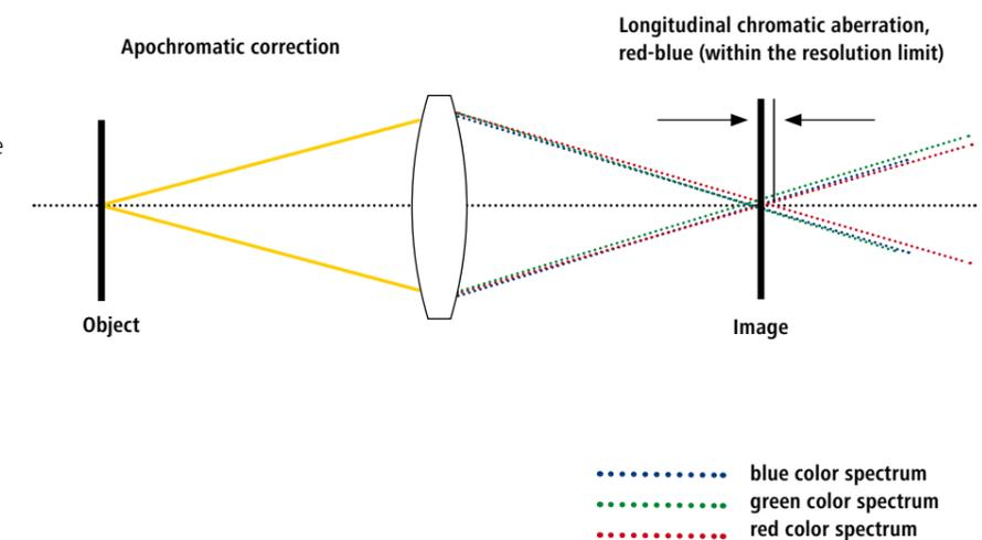
Figure 1.15: When white light passes through a lens, it is broken into its spectral components. Blue light is refracted more than red and thus focuses closer to the lens. Therefore, there is no single focal point for all colors. After apochromatic correction, the different colour components of light are nearly focused at a single point. The result is brilliant image quality without visible chromatic aberration.
