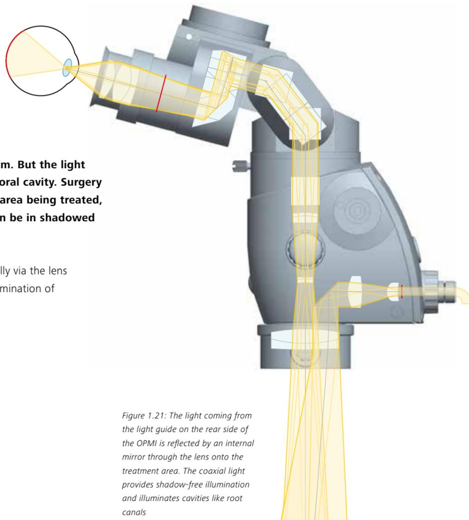
Figure 1.21: The light coming from the light guide on the rear side of the OPMI is reflected by an internal mirror through the lens onto the treatment area. The coaxial light provides shadow-free illumination and illuminates cavities like root canals
