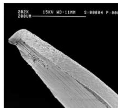
Right: Damaged needle tip after touching the enamel surface of a neighbouring tooth
