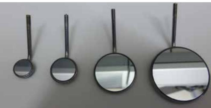
Figure 3.6 Fig HR mirrors in Size 000, 0, 4 and 8
