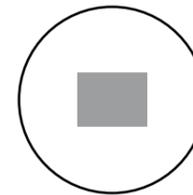
Camera chip size too small in relation to focal length of photo adapter
