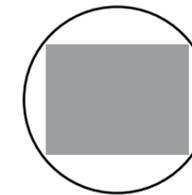
Camera chip size correct in relation to focal length of photoadapter
